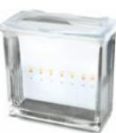
**How it works:** This technique aims to analyze mixtures of chemicals by separating the compounds present. As part of the test, a stationary phase (usually a silica gel) is deposited over a glass or aluminum support, and mixtures of the sample are applied to it. After elution with an organic solvent, the different compounds will move upwards at different rates, allowing their separation.
